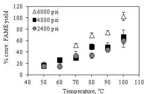
**Figure 4:** FAME yield from wet, frozen algae extracted by scCO<sub>2</sub> across temperature shown as a percentage of the conventional extraction yield for FAME on a per mass basis.
