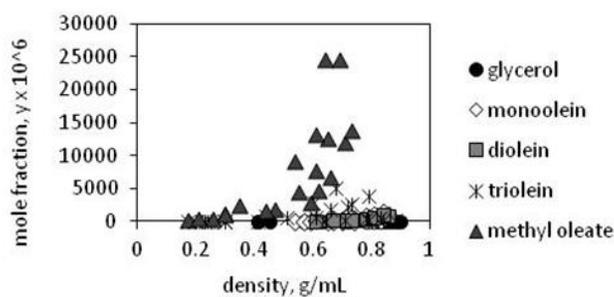
**Figure 3:** Solubility of oleate species in scCO<sub>2</sub>. Data shown as a compilation [39] across density from a range of temperatures and pressures
