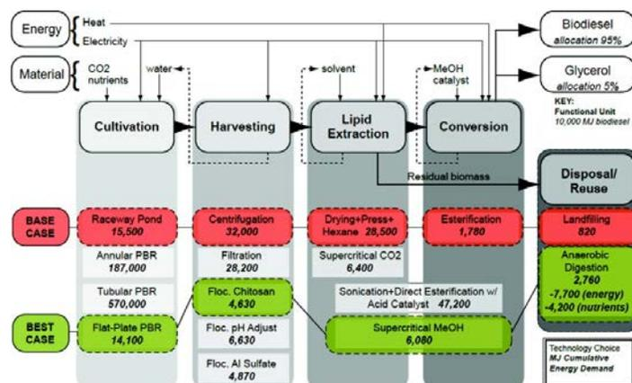
**Figure 1:** Life cycle analysis results of the energy requirements for algal biodiesel production [14].
