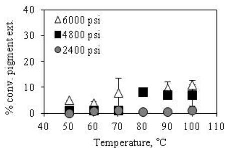
**Figure 5:** Isotherm data for pigment (pheophytin A) extracted with scCO<sub>2</sub> at varying temperature shown as a percentage of extract from conventional solvents.
