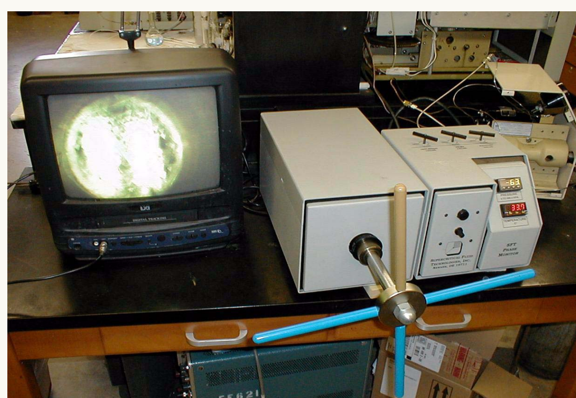
Figure 3. High-pressure view cell apparatus.
