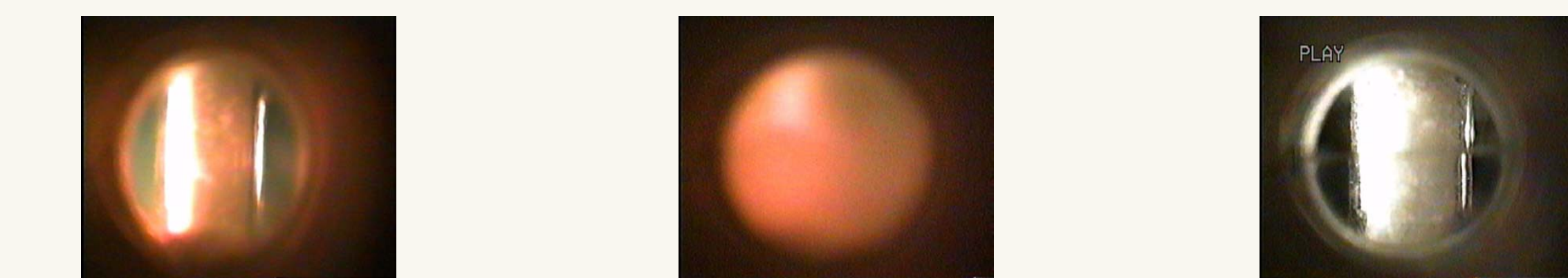
Figure 5. Phase transition of a ternary system from a supercritical state through LCEP to a subcritical state.
