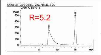
*Figure 3:* Analytical SFC chromatogram with optimized resolution at 30 degrees Celsius. 16.9 µg injection.
