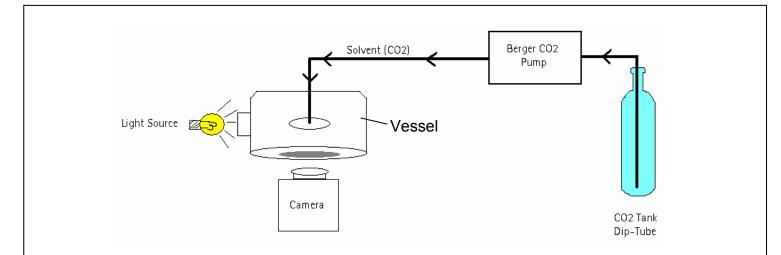
**Figure 1:** General schematic of experimental apparatus, the phase-monitor. Sample would be introduced to the high pressure vessel at various concentrations in the organic modifier volume. Phase monitor modifications were provided through in-house fabrication and control of pressure was accomplished by means of a Berger CO<sub>2</sub> pump. Internal volume of modified vessel is 7 mL.
