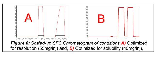
Note the poor peak shape in chromatogram Fig. 6A. Also the quantity
