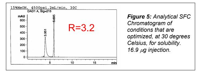
The two methods were run on a Berger Mini-Gram system on a 10x 250 mm, 60A,  $6\mu$  Silica column, with an 200  $\mu$ L loop Alcott autosampler, and Varian Pro-Star detector ( $\lambda$ =250 nm)(Table 2, Figure 6) for comparison.
