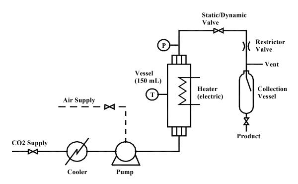
Figure 1: Flowsheet of Supercritical Fluid Extraction Setup
