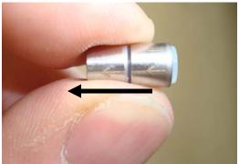
Arrow on Check Valve indicates direction of flow.
